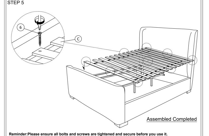
When moving bed position, the center support leg levelers must be adjust up right to avoid breakage of the leg and center support.
